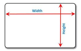
Do not use any cards outside the printer card thickness specification 0.50 - 1.27mm (20 - 50 mil). To do so may result in a card jam or damage within the printer and may not be covered under the manufacturer's warranty.
