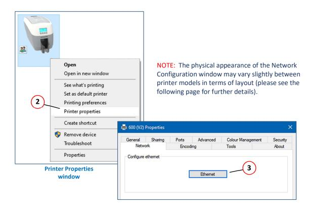
The Network and Configuration window allows the user to set (and store) an IP address in the printer. The user also has the option to choose a static or dynamic IP address. (Static IP settings are generally more commonly used with networked printers).
