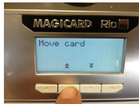
The arrows show the direction that the rollers will rotate when button is pushed
