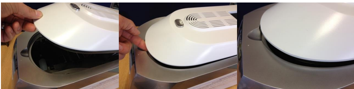
Lower the lid (DO NOT SHUT – lower) This gives easier access to the rear feed roller
