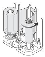
**5** Remove any slack in the laminate film
