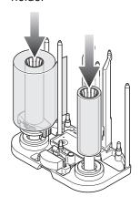
**3** Attach the unused portion at the supply side to the other end at the take-up side using an adhesive tape, while making sure that the joint surface is even
