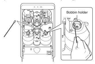
**6** Apply alcohol to a cotton swab (large), and use it to wipe the guide rail (x2) at the back
