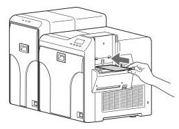
The cleaning card is discharged from the card outlet of the laminator.
