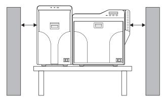
Allow a clearance of at least 10 cm between the rear of the laminator and the wall.
