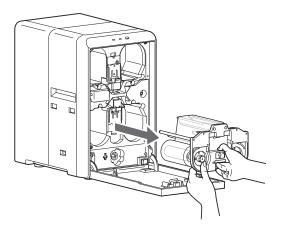
**5** Apply alcohol to a cotton swab (large), and use it to wipe the bobbin holder (x2)
