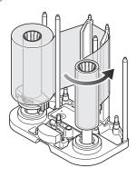
7 Remove any slack in the laminate film
