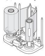
4 Turn the take-up side using your hand until the broken portion can no longer be seen
