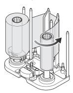
3 Remove any slack in the laminate film
