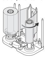
5 Remove any slack in the laminate film
